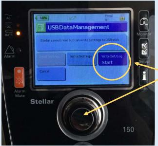
After inserting the USB stick the following window comes up.
