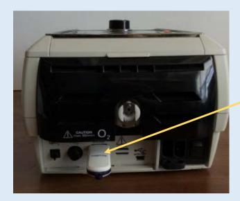
Insert an <u>empty</u> USB stick into either USB port found at the back of the Stellar 150™. Only 1 USB stick can be used at a time.
