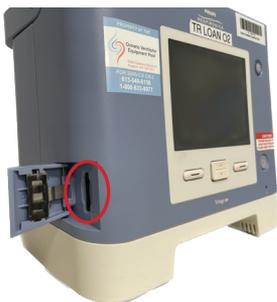
Figure 2. Card in SD card slot
